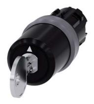
key-operated switch Siemens, 22 mm, round, plastic with metal front ring, lock number SSG10, with 2 keys, 3 switch positions I>O<II, momentary contact on the left, latching on the right, actuating angle 2x45°, 10:30h/12h/13:30h, key removal O+II, with laser labeling, inscription or symbol customer-specific selection with SIRIUS ACT configurator (CIN)
