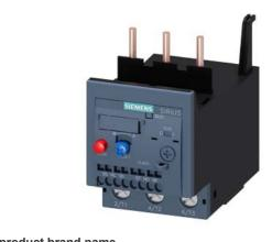
Overload relay 18...25 A Thermal For motor protection Size S2, Class 10 Contactor mounting Main circuit: Screw Auxiliary circuit: spring-type terminal Manual-Automatic-Reset
