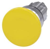
Mushroom pushbutton, 22 mm, round, metal, shiny, yellow, 40 mm, momentary contact type, with laser labeling, upper case and lower case, always upper case at the beginning of the word
