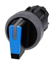
Selector switch, illuminable, 22 mm, round, plastic with metal front ring, blue, selector switch, short, 3 switch positions I>O<II, momentary contact type, actuating angle 2x45°, 10:30h/12h/13:30h, Z=50-unit packaging
