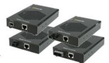
The S-1110P-XT Industrial Temperature PoE Media Converters address the need for transparently connecting 10/100/1000 Ethernet equipment that operate in extreme temperatures to fiber while providing Power over Ethernet ( PoE ) to standards-based PoE and PoE+ compliant devices.
