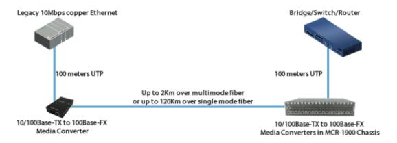
10/100 - Extend Network between Half-Duplex Hubs
