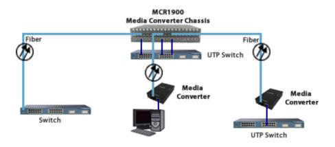
10/100 - Extend Network between Ethernet Hubs
