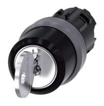
RONIS key-operated switch, 22 mm, round, plastic with metal front ring, lock number SB30, with 2 keys, 3 switch positions I>O<II, momentary contact on the left, latching on the right, actuating angle 2x45°, 10:30h/12h/13:30h, Key removal O+II, possible special locks: SB31, 421, 455, with laser labeling, upper case and lower case, always upper case at the beginning of the word
