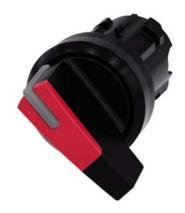
Selector switch, illuminable, 22 mm, round, plastic, red, selector switch, long, 2 switch positions O-I, latching, actuating angle 90°, 10:30h/13:30h, with laser labeling, upper case and lower case, always upper case at beginning of line
