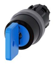
Key-operated switch O.M.R, 22 mm, round, plastic with metal front ring, lock number 73038, blue, with 2 keys, 3 switch positions I-O-II, latching, actuating angle 2x45°, 10:30h/12h/13:30h, key removal O, with laser labeling, upper case and lower case, always upper case at beginning of line
