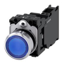
Illuminated pushbutton, 22 mm, round, Metal, shiny, blue, pushbutton, flat, momentary contact type, with holder, 1 NO+1 NC, LED module with integrated LED 230 V AC, spring-type terminal, with laser labeling, upper case and lower case, always upper case at the beginning of the word
