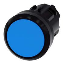
Pushbutton, 22 mm, round, plastic, blue, pushbutton, flat momentary contact type, with laser labeling, symbol number according to, ISO 7000 or IEC 60417
