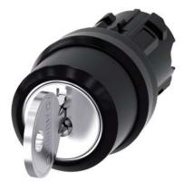
RONIS key-operated switch, 22 mm, round, plastic, special lock, with 2 keys, 3 switch positions I>O<II, momentary contact type, actuating angle 2x45°, 10:30h/12h/13:30h, key removal O, possible special locks: SB31, 421, 455
