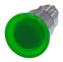
Illuminated mushroom pushbutton, 22 mm, round, metal, shiny, green, 40 mm, 3 switch positions, latches after pushing in, unlatches by pull-to-unlatch mechanism to center position, after pulling out the button Retraction to center position, with laser labeling, lower case
