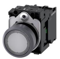
Illuminated pushbutton, 22 mm, round, plastic with metal front ring, clear, pushbutton, flat, momentary contact type, with holder, 1NO, LED module with integrated LED 24 V AC/DC, screw terminal, with laser labeling, upper case
