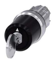
Key-operated switch BKS, 22 mm, round, metal, shiny, lock number S1, with 2 keys, 3 switch positions I>O<II, momentary contact type, actuating angle 2x45°, 10:30h/12h/13:30h, key removal O, with laser labeling, lower case
