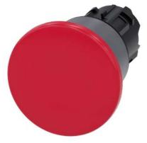
Mushroom pushbutton, 22 mm, round, plastic with metal front ring, red, 40mm, latching, pull-to-unlatch mechanism, with laser labeling, symbol number according to, ISO 7000 or IEC 60417
