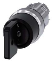
Key-operated switch O.M.R, 22 mm, round, metal, shiny, lock number 73034, black, with 2 keys, 3 switch positions I>O<II, momentary contact type, actuating angle  $2x45^{\circ}$ , 10:30h/12h/13:30h, key removal O, with laser labeling, upper case and lower case, always upper case at the beginning of the word
