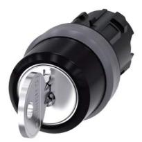
RONIS key-operated switch, 22 mm, round, plastic with metal front ring, lock number SB30, with 2 keys, 3 switch positions I-O-II, latching, actuating angle 2x45°, 10:30h/12h/13:30h, Key removal I+II, possible special locks: SB31, 421, 455, with laser labeling, upper case and lower case, always upper case at the beginning of the word
