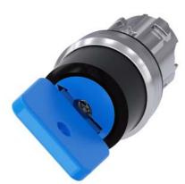
Key-operated switch O.M.R, 22 mm, round, metal, shiny, lock number 73038, blue, with 2 keys, 2 switch positions O-I, latching, actuating angle 90°, 10:30h/13:30h, key removal O+I, with laser labeling, lower case
