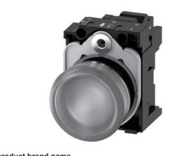
Indicator lights, 22 mm, round, metal, shiny, clear, lens, smooth, with holder, LED module with integrated LED 110 V AC, spring-type terminal, with laser labeling, upper case and lower case, always upper case at the beginning of the word
