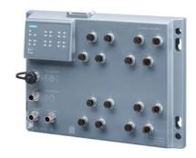
SCALANCE XP216EEC, managed IE switch, with railway approval IEC 62443-4-2 certified; (EN 50155, EN45545); 12x 10/100 Mbit/s M12 ports, 4x 10/100/1000 Mbit/s M12 ports IP65, LED diagnostics, error signaling contact, redundant power supply, PROFINET IO device, network management, can be operated in redundant ring, incl. dust caps, including electronic manual on CD-ROM, C-PLUG optional.
