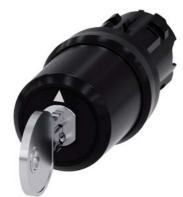
Key-operated switch BKS, 22 mm, round, plastic, lock number S1, with 2 keys, 3 switch positions I>O<II, momentary contact type, actuating angle 2x45°, 10:30h/12h/13:30h, key removal O, with laser labeling, upper case
