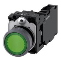
Illuminated pushbutton, 22 mm, round, plastic with metal front ring, green, pushbutton, flat, momentary contact type, with holder, 1 NO+1 NC, LED module with integrated LED 110 V AC, screw terminal, with laser labeling, upper case and lower case, always upper case at beginning of line
