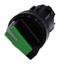
Selector switch, illuminable, 22 mm, round, plastic, green, selector switch, short, 2 switch positions O<I, momentary contact type, Actuating angle 45°, 10:30h/12h, with laser labeling, inscription or symbol Customer-specific selection with SIRIUS ACT configurator (CIN)
