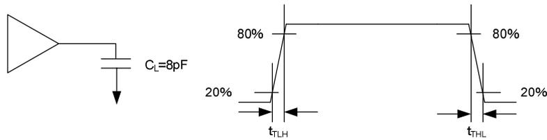
Figure 8. LVC MOS Output Load and Transition Time
