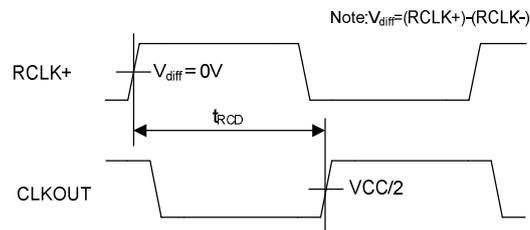
Figure 10. Input Clock to Output Clock Delay Time
