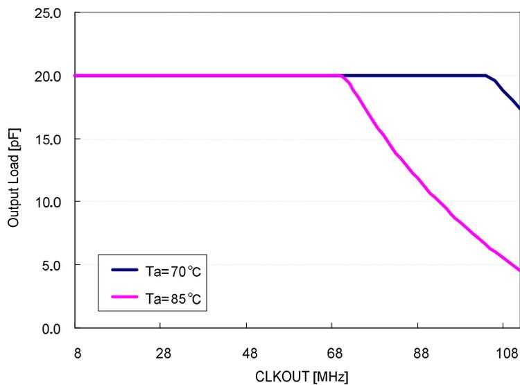
**Figure 6. LVC MOS Output Load Limitation**
